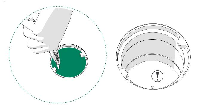
**4.** Drill a pilot hole through the ceiling felt from above.
