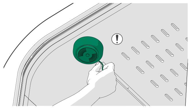
6. Guide the electrical wiring out of the notch in the roof.
