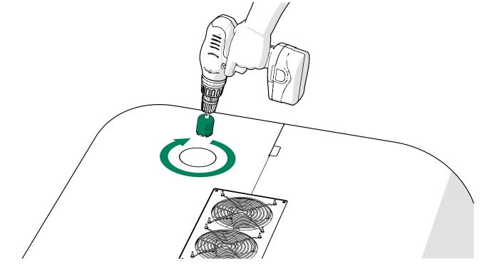
5. Cut out a hole in the ceiling felt for the sprinkler head from the inside of the pod. You can use a hole saw or utility knife. If you use a hole saw, chose the size according to the size of the sprinkler head.
